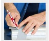
Wrap the tape once around the roller at the desired angle and mark the point where the end of the roll meets the second turn of the tape.
