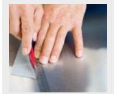
Put the tape on a flat surface and cut it diagonally from the end of the roll to the marked point of the tape.
