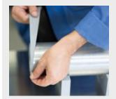
Remove the liner and start applying the tape, starting from the edge of the roller.
